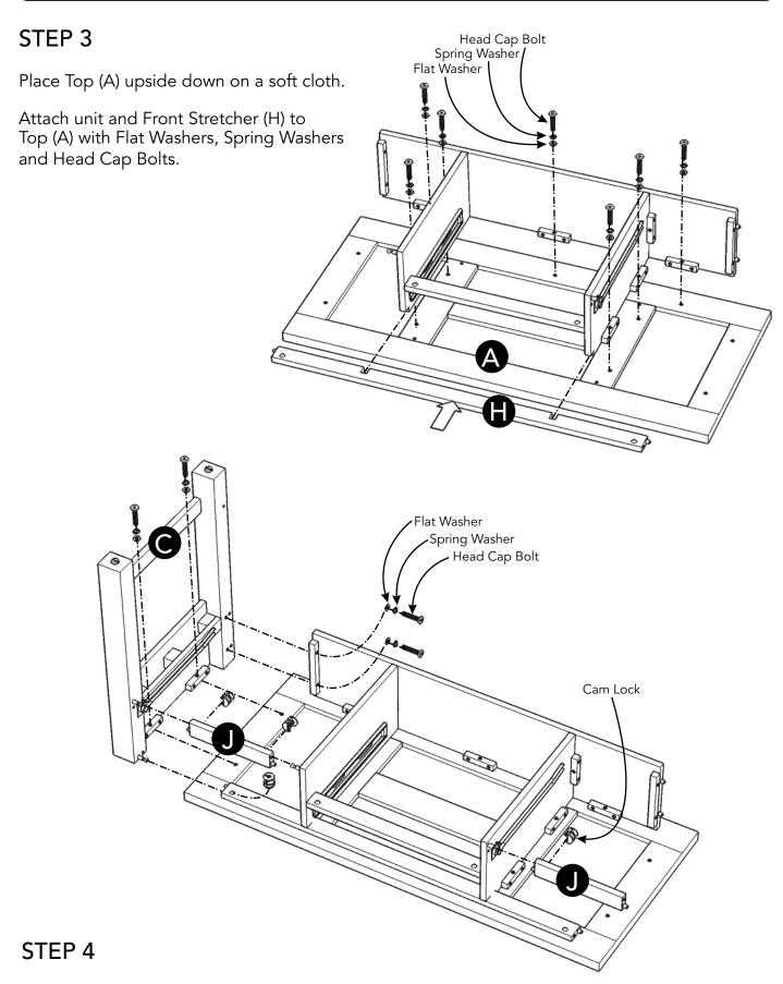
Attach Front Stretchers (J) to unit with Cam Locks.
