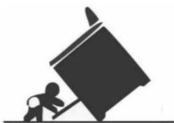
A Child or adult can tip the range which can result in serious injuries or death. Install the anti-tip device to the range and/or structure per installation instructions. Engage the range to the Anti-tip device installed to the structure. Re-engage the anti-tip device if the range is removed. Failure to follow these instructions can result in death or serious injuries and/or burns to children and adults.
