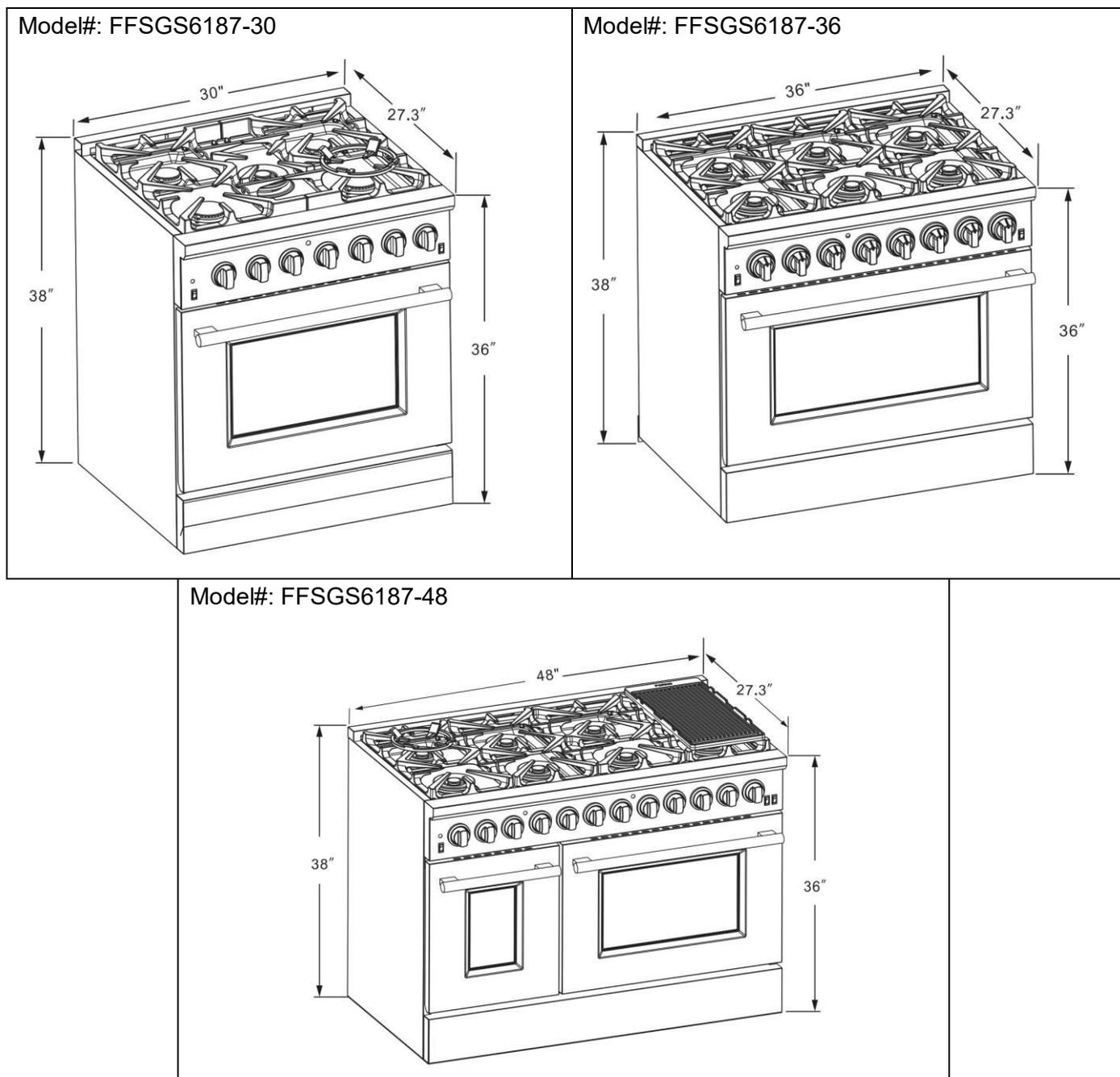
This range may be installed directly adjacent to existing countertop-height cabinets (36" or 91.5 cm from the floor). To achieve the best look, the cooktop should be level with the cabinet countertop. This can be accomplished by raising the unit using the adjustment spindles on the legs.
