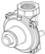
Pressure regulator can withstand a maximum input pressure of 0.5 psi (3.5 kPa), and is set at 5" wc out let pressure.
