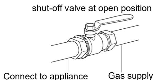
The supply line must be equipped with an approved external gas shut-off valve located near the range in an accessible location. Do not block access to the shut-off valve. Refer to the illustration below.
