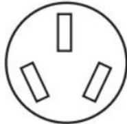
3-wire receptacle (10-50R)
