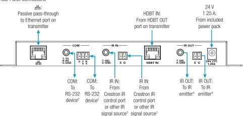
**NOTE:** Connection of the included power pack to the receiver powers both the receiver and the transmitter. Power is transmitted over the cable that connects the HDBT IN port of the receiver to the HDBT OUT port of the transmitter.
