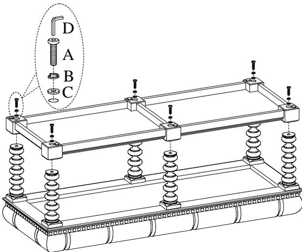
**STEP 2:** Attach the bottom shelf to the legs by using 6 bolts(A), lock washers(B) and flat washers(C). Turn the bench to the upright position.
