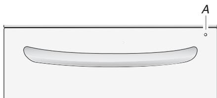
For controls on top of door, the single indicator light (A) on the front of the door panel will remain blue during wash/rinse, red during dry, and white when complete.
