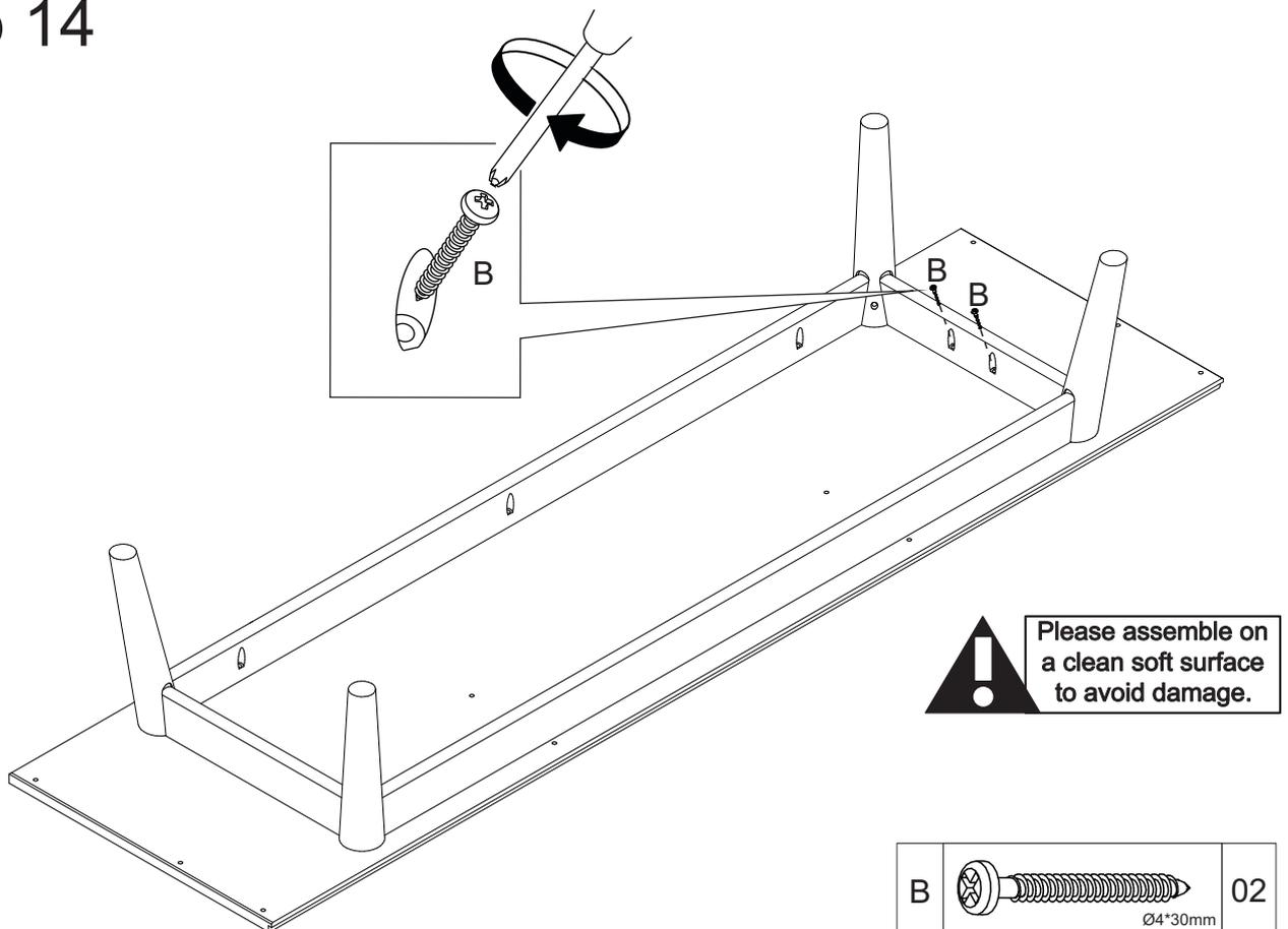
Attach the assembled part to the base (26) using screw (B) and Phillips head screwdriver.
