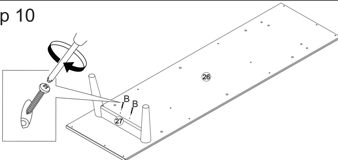
Attach the assembled part to the base (26) using screw (B) and Phillips head screwdriver.
