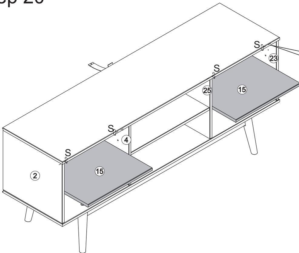
Insert the accessory (S) into the holes in the parts (2), (4), (23) and (25).
