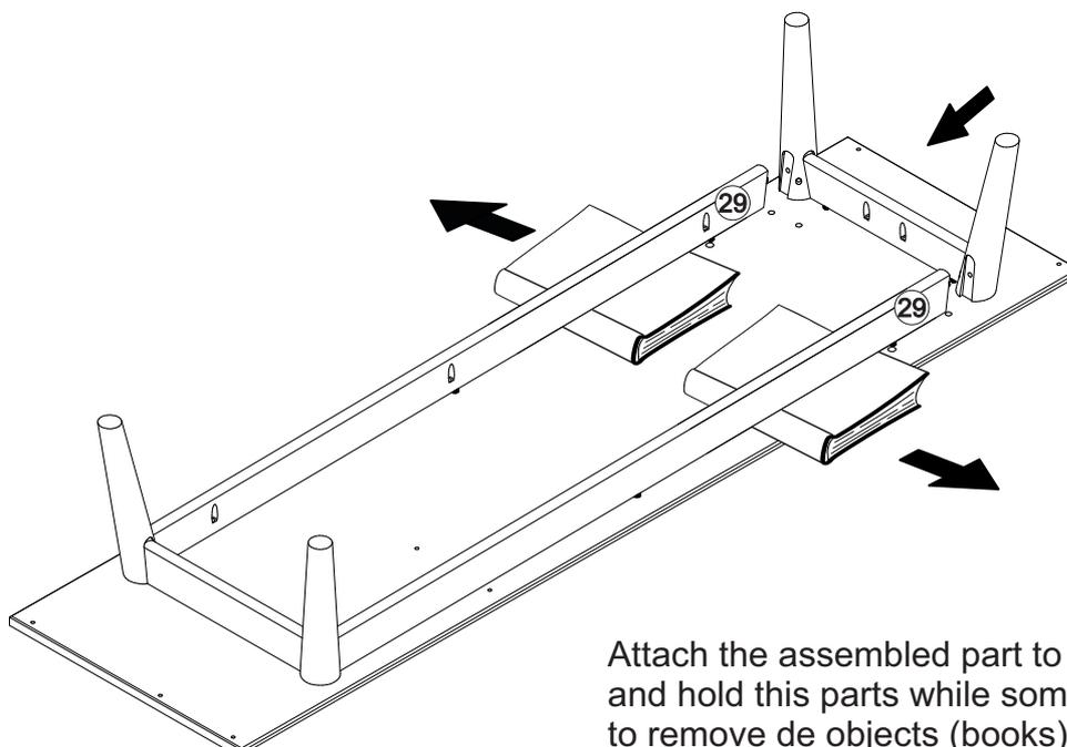
Attach the assembled part to the parts (29) and hold this parts while someone help to remove de objects (books).
