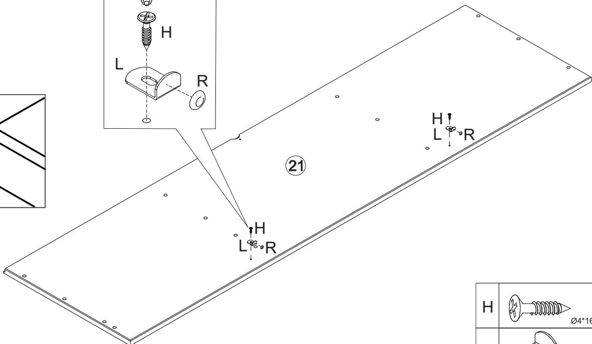
Attach the accessory (R) to the accessory (L), then secure everything to the part (21) with a screw (H) and a Phillips screwdriver.
