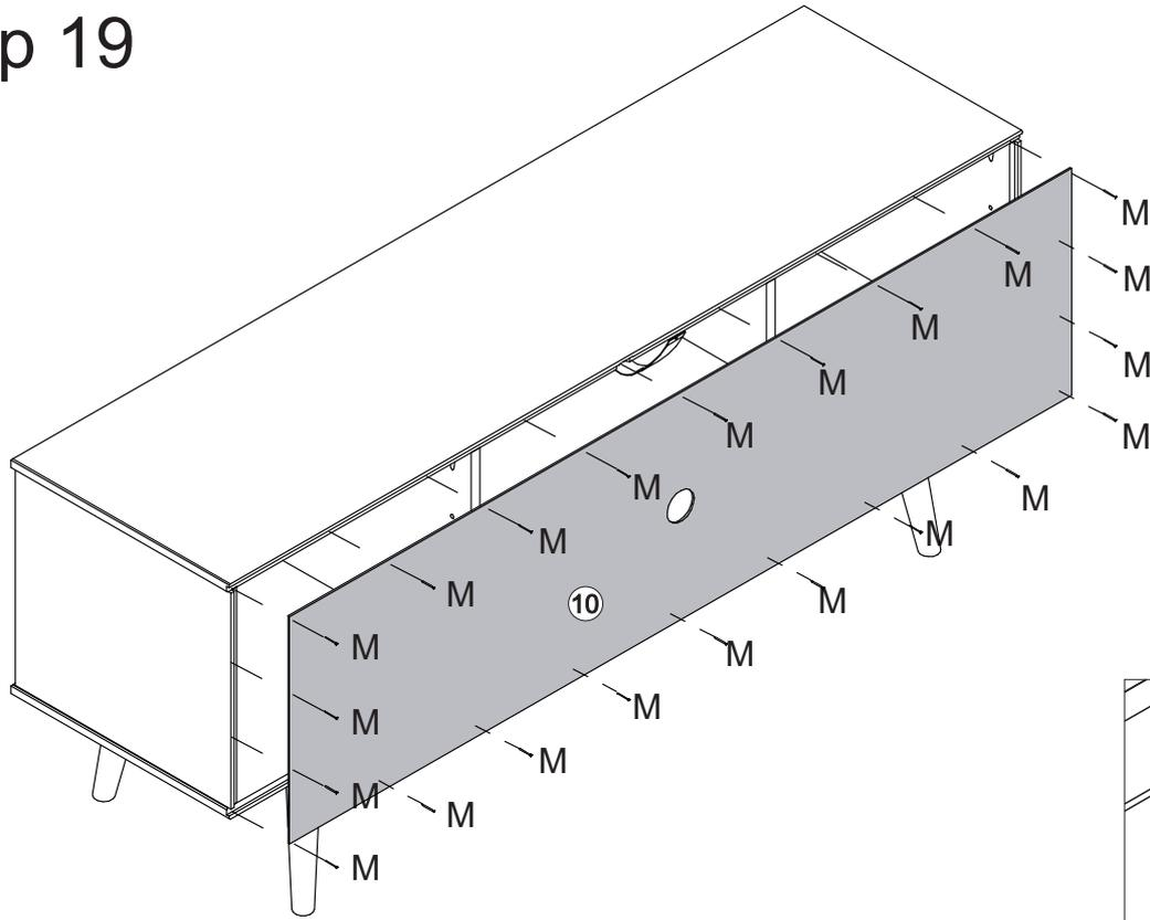
Secure back panel (10) to body with nails (M) and hammer.
