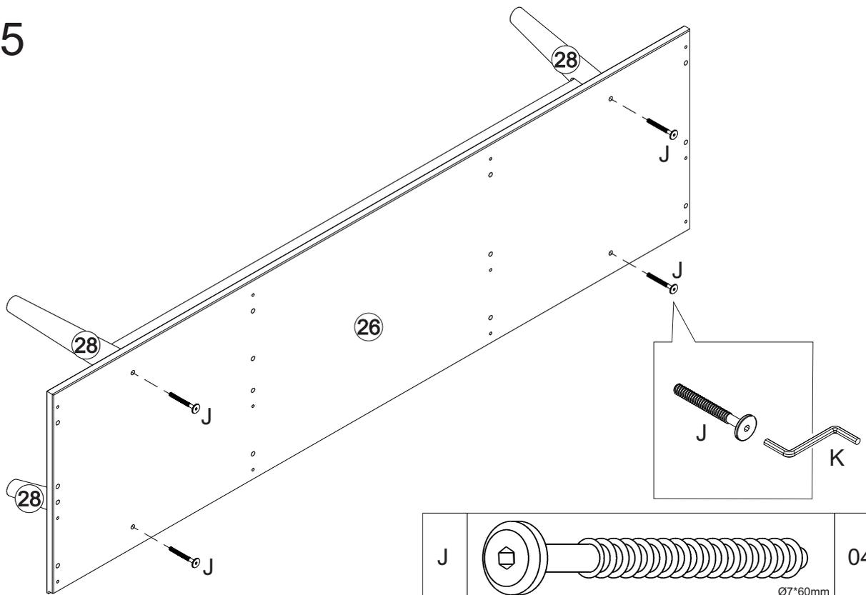
Attach the foot (28) to the base (26) using screw (J) and hex key (K).
