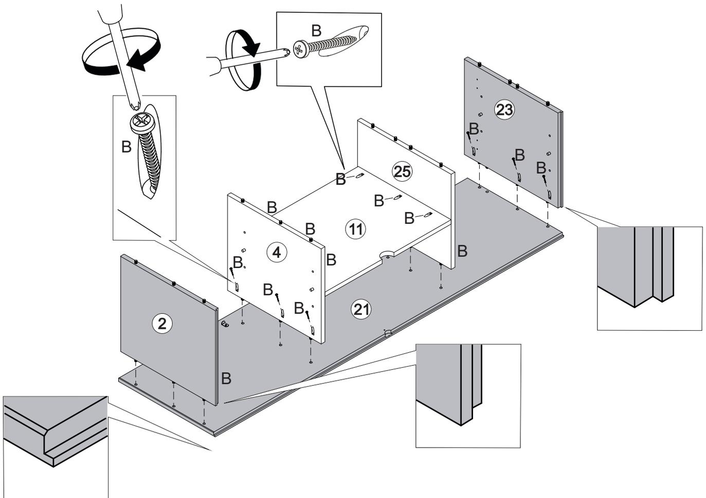
Secure part (2), (4), (23) and (25) to part (21) with screw (B) and a Phillips screwdriver.
