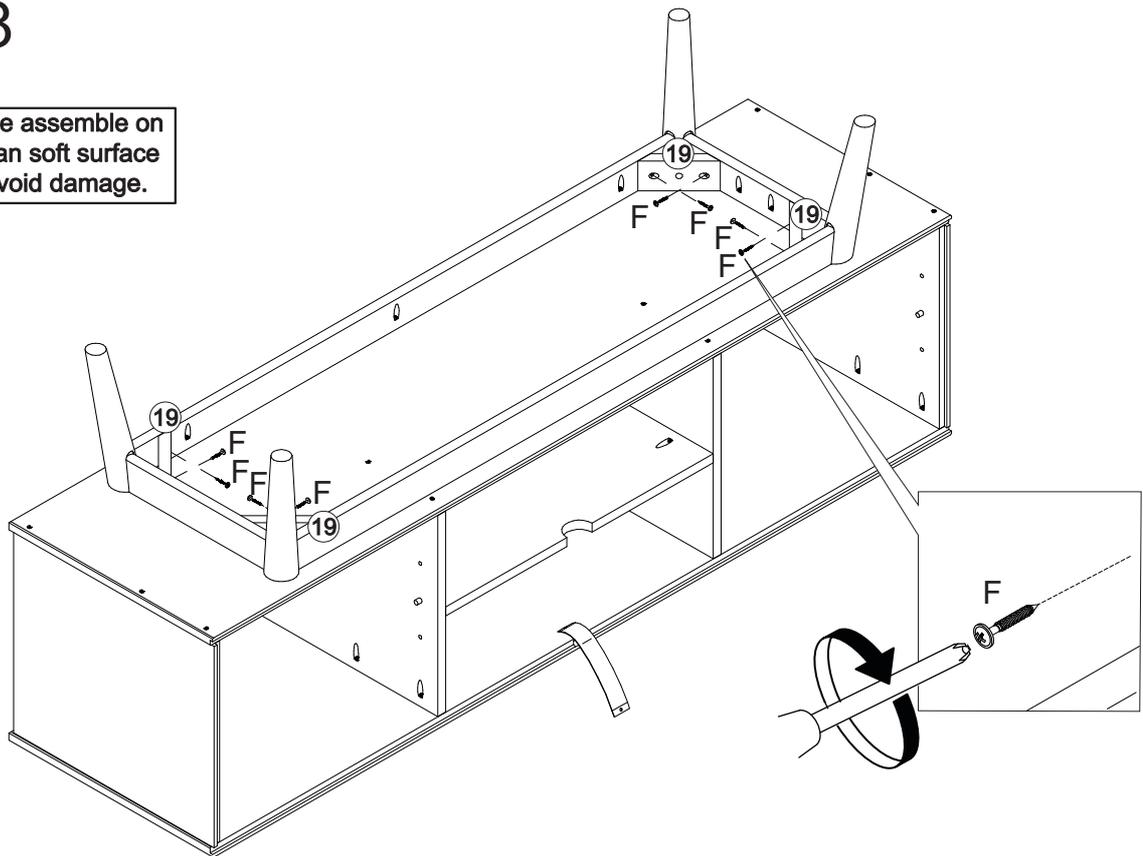
Fix the parts (19) to the body using the screw (F) and Phillips screwdriver.
