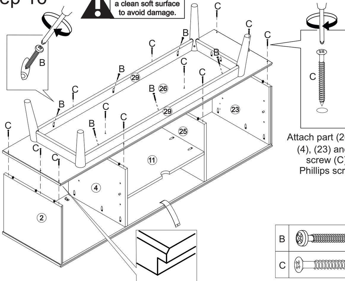
Attach part (26) to parts (2), (4), (23) and (25) using screw (C) and a Phillips screwdriver.
