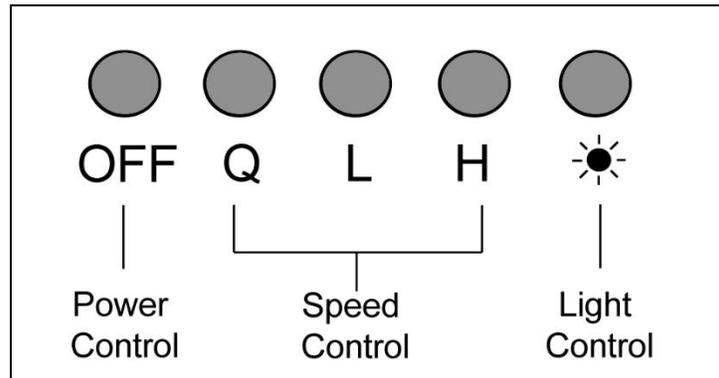
NOTE: For best result, turn fan on prior to any preparation or cooking and keep fans running while cooking. Adjust speed as necessary.
