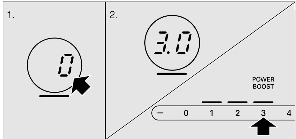
3. Changing the heat setting: Select the element and change the heat setting with the 1 to 9 symbols or the + and – symbols.
