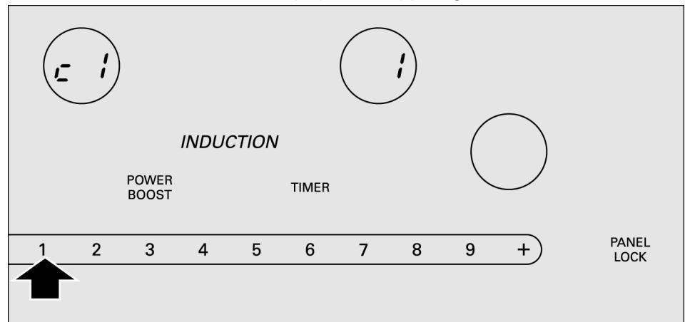
5. Press the **PANEL LOCK** symbol again for more than 4 seconds, until you hear a sound signal. The settings have been correctly stored.
