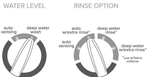
Set the Water Level knob to the Auto Sensing setting and the washer will automatically sense the appropriate water level for the load size and type.
