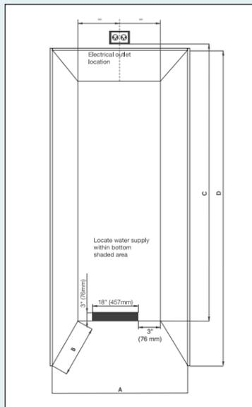
\*The given cabinet opening height dimension includes space for top air vent. If you choose to place the vent above the cabinet or in a soffit, you will need to adjust the height dimensions accordingly. Please refer to Ventilation Requirements.
