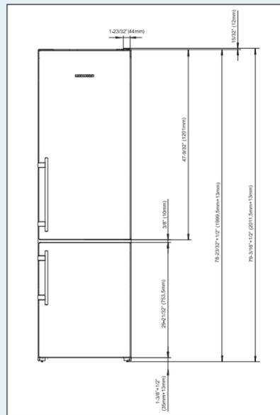
When installing CS units into a row of cabinets or wall units: Use these dimensions to achieve a custom look with the cabinetry while providing the necessary clearance for the top door hinge.
