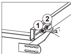
b) The headboard bracket has 2 adjustable slots to accommodate any frame type. Use the bolts and washers to secure the bracket. Make sure the bolts are tight.
