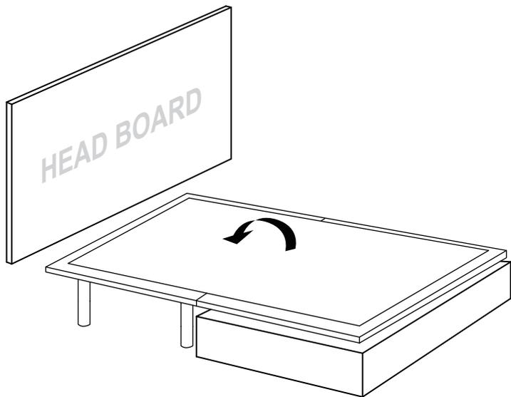
**7** Flip the foot end of the bed from the box and lay it on top of the end at the headboard.
