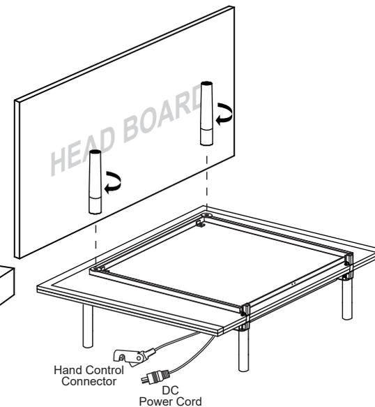
**9** Connect the hand control and secure it with the connector lock. Uncoil the AC power cord, connect the DC power cord to the power supply.
