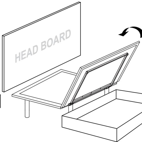
**8** Install the remaining 2 legs on the foot end of the bed, make sure the legs are tight. Uncoil the DC power cord and the hand control connector.
