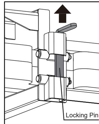
**5** Attach the 1.6" leg section to 11.3" section. The (2) legs will be installed on Step 8.
