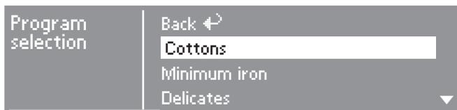
You can use the multi-function selector to select any program. The highlighting will move up or down depending on the direction the multi-function selector is turned in.
