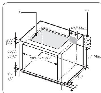
\* See built-in oven installation for complete installation instructions. See label on top of approved built-in oven models.
