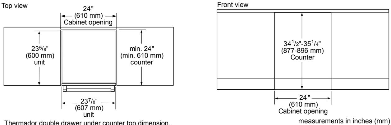
Thermador double drawer under counter top dimension. (Unit door flushed with the cutout) measurements in inches (mm)
