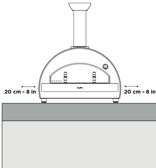
**CAUTION!** When being used, place the oven at a safe distance from flammable materials or substances that may be damaged by heat.
