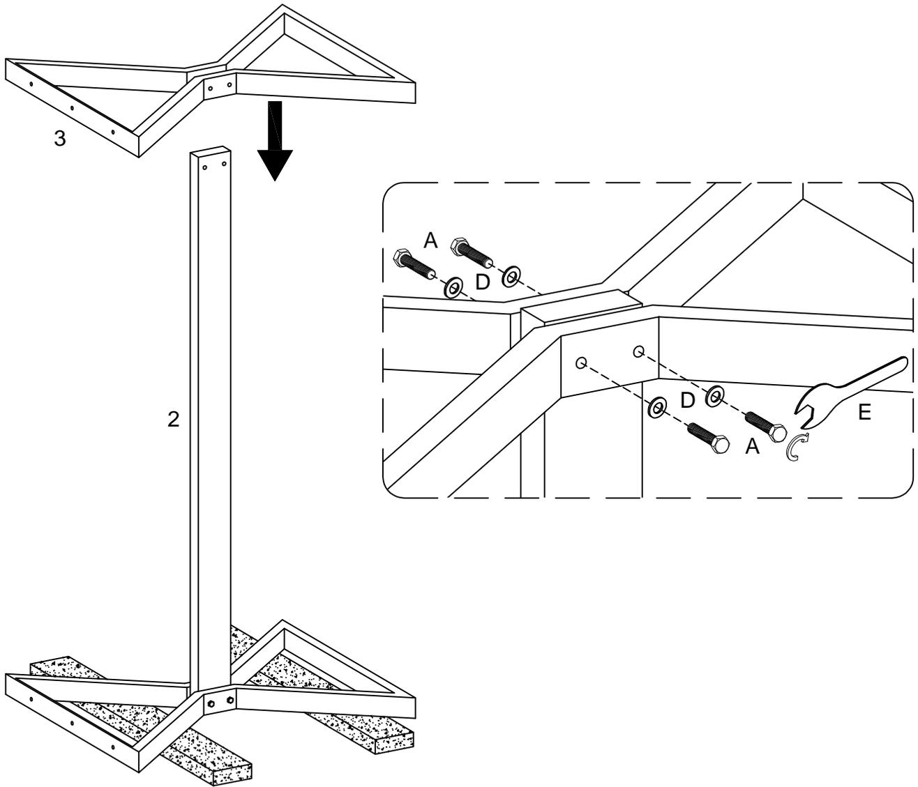
Place part (3) to part (2) ,then using bolt (A) attach flat washer (D) into part (3) to part (2) with wrench (E) as per diagram.
