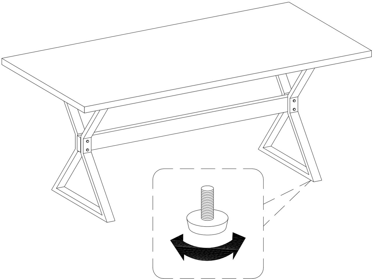
Position the assembled unit at the desired location ,if necessary adjust the floor leveler at the bottom of the leg to level the unit .
