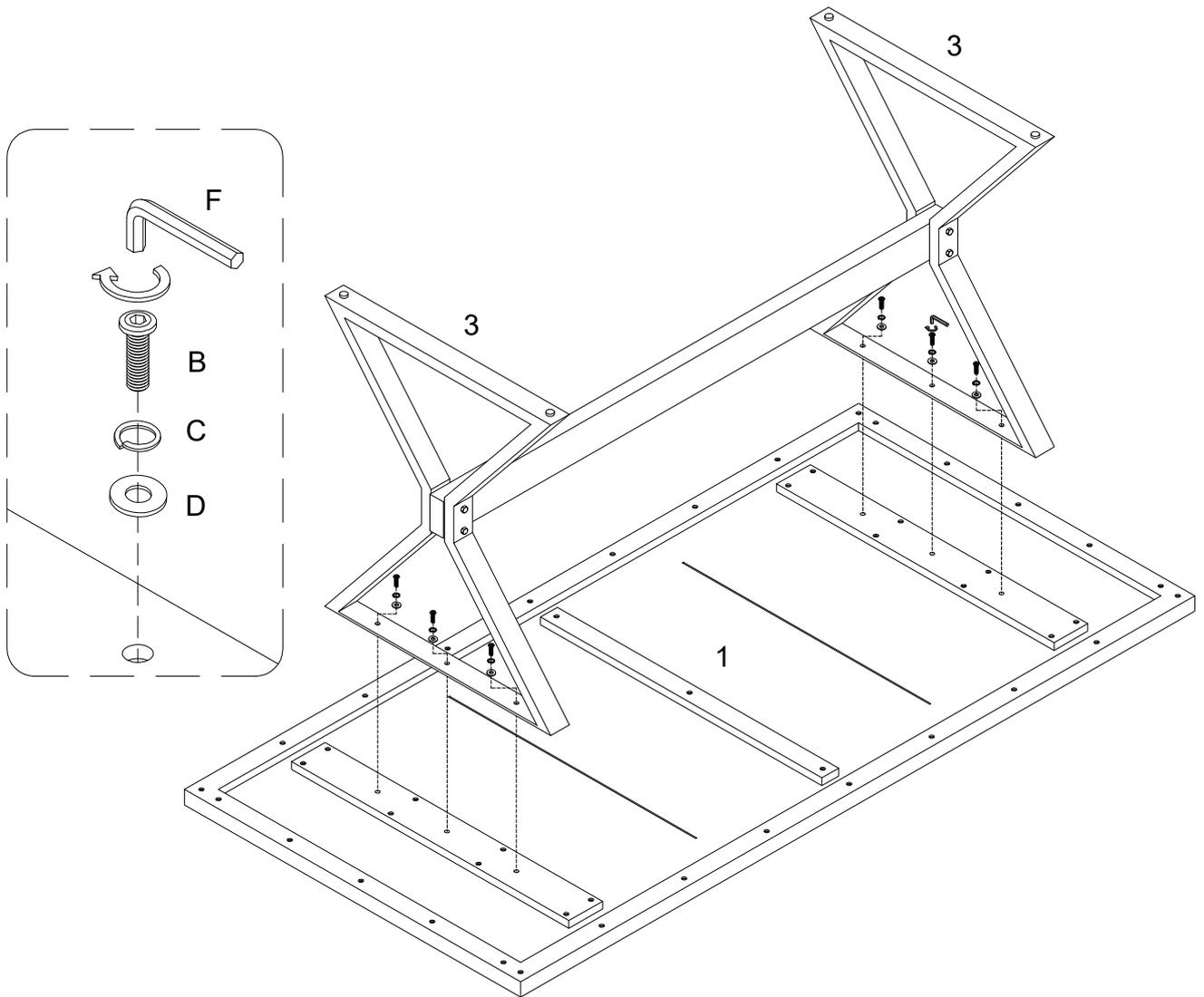
Using bolt (B) attach Lock washer (C) and Flat washer (D) into part (3) to part (1) with Hex key (F) as per diagram.
