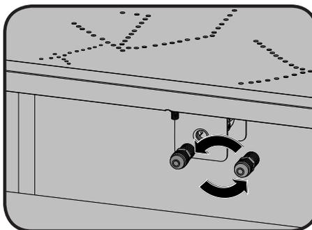
5. Replace the propane orifice with the natural gas orifice supplied.
