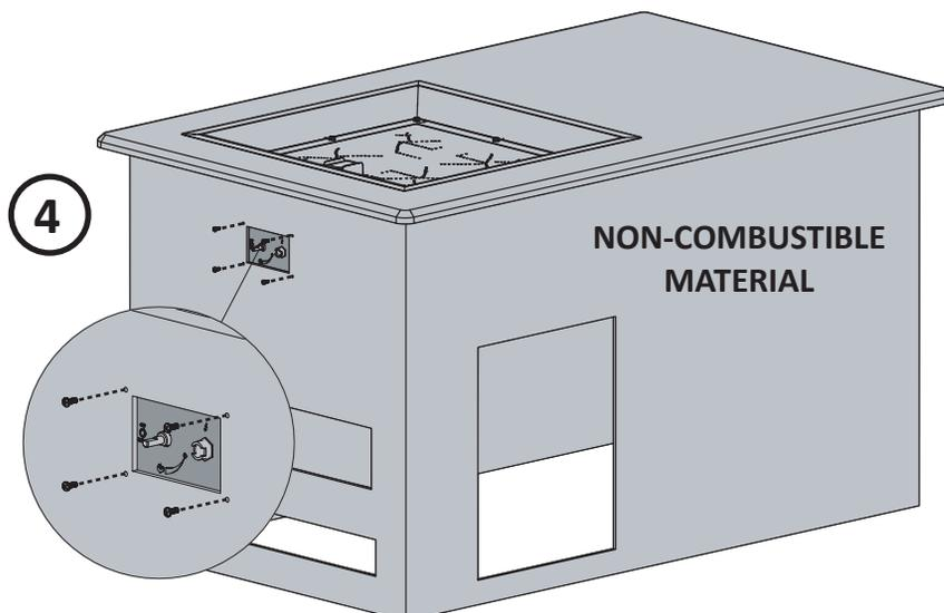
Center of valve must be a minimum of 8" (203mm) below the top surface of burner.
