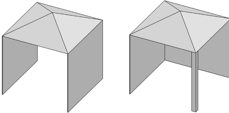
Within a partial enclosure which includes an overhead cover and three sidewalls, as long as 30 percent or more of the horizontal periphery of the enclosure is permanently open.
