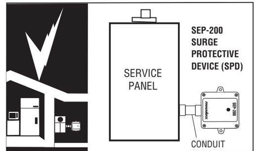
*For use before or after the main disconnect for optimum lightning protection.*
