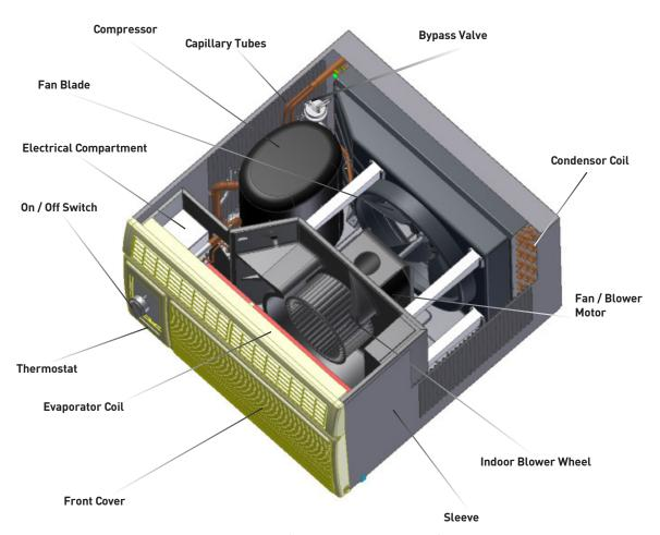
Figure 101 (Component Identification)
