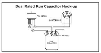
Figure 506 Dual Rated Capacitor Hook-Up
