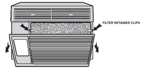
The filter can be removed for cleaning by opening the front of the unit and releasing the filter from its retaining clips.
