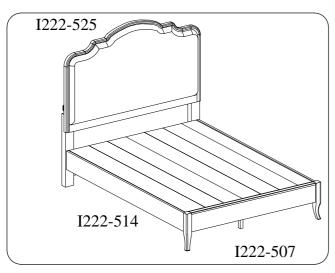
All Beds need to be set up in the exact final location so that after full assembly it will not need to be moved. Moving the bed will cause the support legs to move out of perpendicular (90 degree), weaken the support system, and may allow the bed to collapse.
