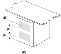
If the front of the appliance is covered, louvered openings must be installed as shown and front/rear clearances adhered to according to closet installations.
