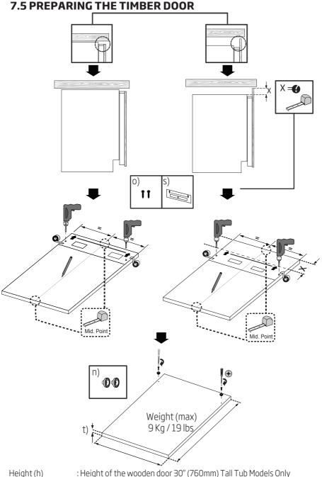
Height (h) : Height of the wooden door 30" (760mm) Tall Tub Models Only Height (h) : Height of the wooden door 28" (720mm) Standart Tub Models Only
