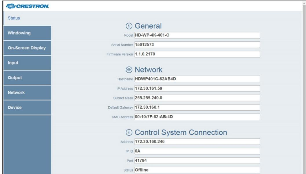
The screenshot shows the Crestron web interface for the HD-WP-4K-401-C. On the left is a navigation bar with the following items: Status, Windowing, On-Screen Display, Input, Output, Network, and Device. The main content area is titled 'Status' and contains three sections:
