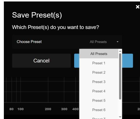
Save configured parameters to a specific Preset (e.g., Preset 1), or save all configured Presets collectively into a single Preset file (All Presets).
