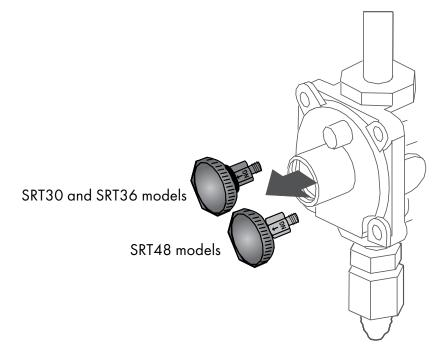
• Remove the regulator pin by pulling it out (see figure above). For SRT30 and SRT36 models, the pin will be gray in color. For SRT48 models, the pin will be gold.
