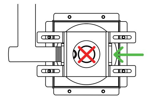
Refer to this diagram for proper gas hookup on the right side of the regulator.
