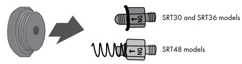
• Unscrew the retainer pin, reverse it, and screw back into the regulator cap as outlined in the figures above and below. For SRT30 and SRT36 models, the gray pin is not attached to a spring. For SRT48 models, the gold pin is attached to a spring. When reversing the SRT48 pin, ensure the spring is snug when tightening.
