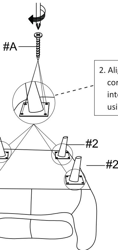
2. Align the legs (#2) to each corner then insert 4 screws (#A) into each leg (#2). Secure using a Phillips screwdriver.
