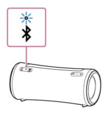
After you pair the speaker with a BLUETOOTH device for the first time since purchase or initialize the speaker (the speaker has no pairing information), the speaker automatically enters pairing mode when it is turned on. Proceed to step
