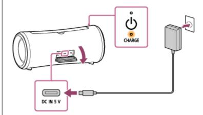
Battery charging starts and the CHARGE indicator lights up in orange. Charging will complete in about 5 hours<sup>\*</sup> and the indicator will turn off.
