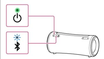
When the speaker has no pairing information, for example when you use the BLUETOOTH function for the first time after purchase, the **\*** (BLUETOOTH) indicator keeps double flashing in blue.
