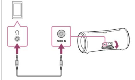
\*1 If you use an audio cable (with stereo mini plugs) with significant resistance, the sound may be lower. Therefore, make sure you use a cable (with stereo mini plugs) without resistance.
