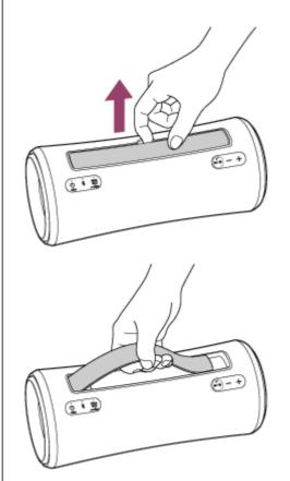
**2** Push in the middle section of the handle to retract the handle.
