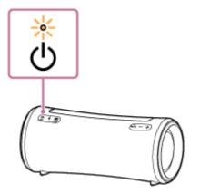
When an abnormality of the built-in battery has been detected, stop charging immediately, wait for a while, and then charge the built-in battery again. If the problem persists, contact your nearest Sony dealer.
