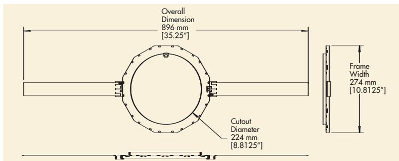
**Specifications:** Grille Diameter 9 3/4" (24.76 cm); Cutout Diameter 8 3/4" (22.2 cm); Total Depth \*3 3/8" (9.77 cm); Mounting Depth In Wall \*\*3 3/8" (8.5 cm); Woofer 8" (20 cm); Tweeter 1" (25 mm); Product Weight 4.8 lb. (2.14 kg); Frequency Response 26 Hz – 30 kHz; Sensitivity 90 dB; Impedance compatible with 4 – 8 Ohm outputs; Min/Max Recommended Power 10/225 WPC
