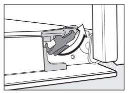
Release the locking clamps by turning them as far as they will go. Do not attempt to take the door off the brackets when it is in the horizontal position, the brackets will spring back against the oven.
