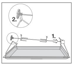
Insert the pointed end of the rotisserie (1.) into the motor slot at the back of the rotisserie set up and set the other end onto the holder (2.) as illustrated.
