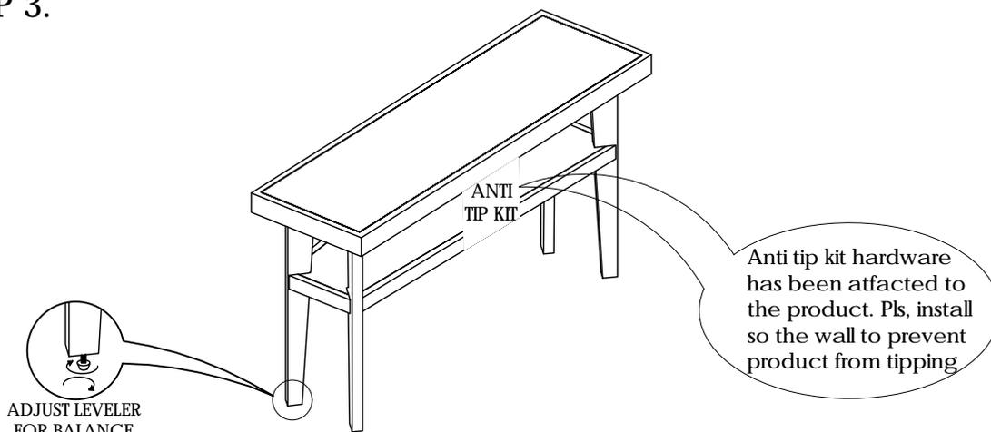
Anti tip kit hardware has been attached to the product. Pls, install so the wall to prevent product from tipping
