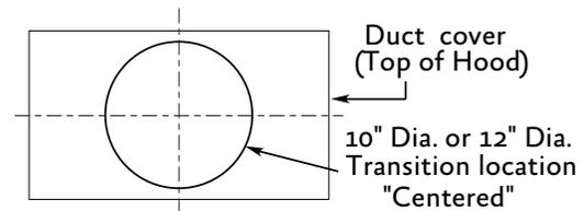
For 900 and 1200 CFM hoods, the transition (AKVT6810 or AKVT8812) is installed in the hood at the factory as a standard item. It will be located in the exact center of the duct cover (left to right & front to rear).
