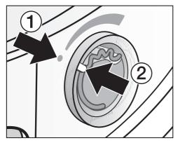
■ Turn the outer ring counterclockwise until markers ① and ② line up.
