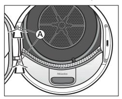
Screw the door securely to the dryer at the base of door hinge A. Now that you have changed the door hinging, the door will open from the opposite side.
