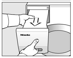
Remove the condensed water container.
