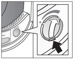
Open the cover using the tab until the tab is at the top right-hand side as shown.
