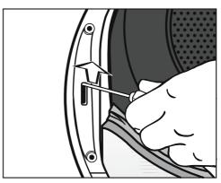
Use the screwdriver to press the door lock upwards.
