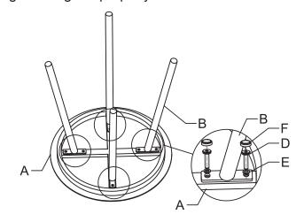
2 Pls secure screw all the bolts are tightened completely, four for each leg, totally 18pcs bolts, if you find the bolts can not be screwd tightenly ,pls return the table.
