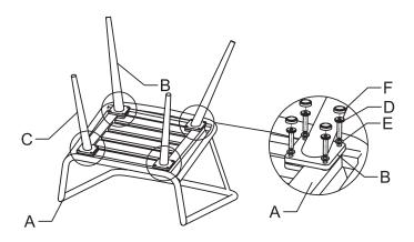
2 Pls secure screw all the bolts are tightened completely, four for each leg, totally 16pcs bolts, if you find the bolts can not be screwd tightenly, pls return the chair.
