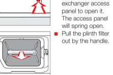
A guide pin in the dryer will come out which prevents the access panel from closing without the plinth filter.
