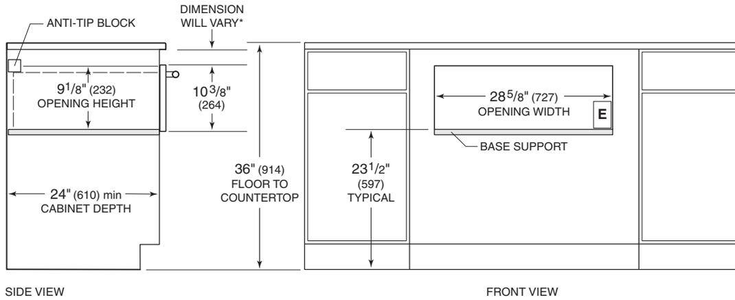
\*Dimension must accommodate height of anti-tip block and drawer face overlap.
