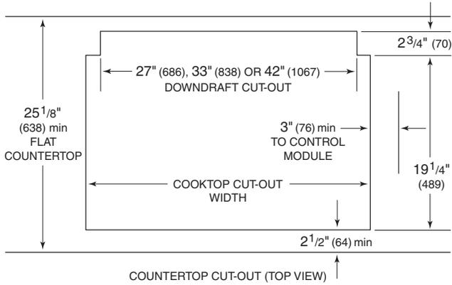
**INSTALLATION WITH SEALED BURNER RANGETOP**
