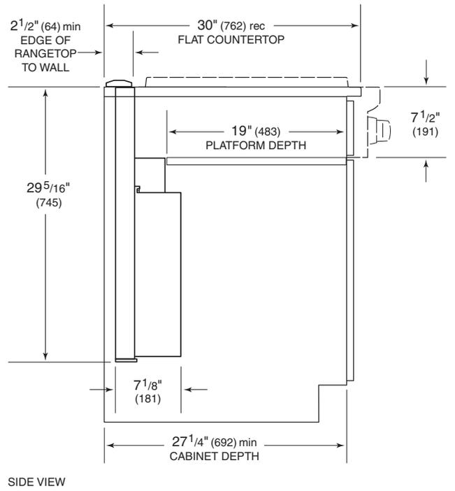
\*Additional depth may be required if rangetop is to be installed flush with cabinet face.
