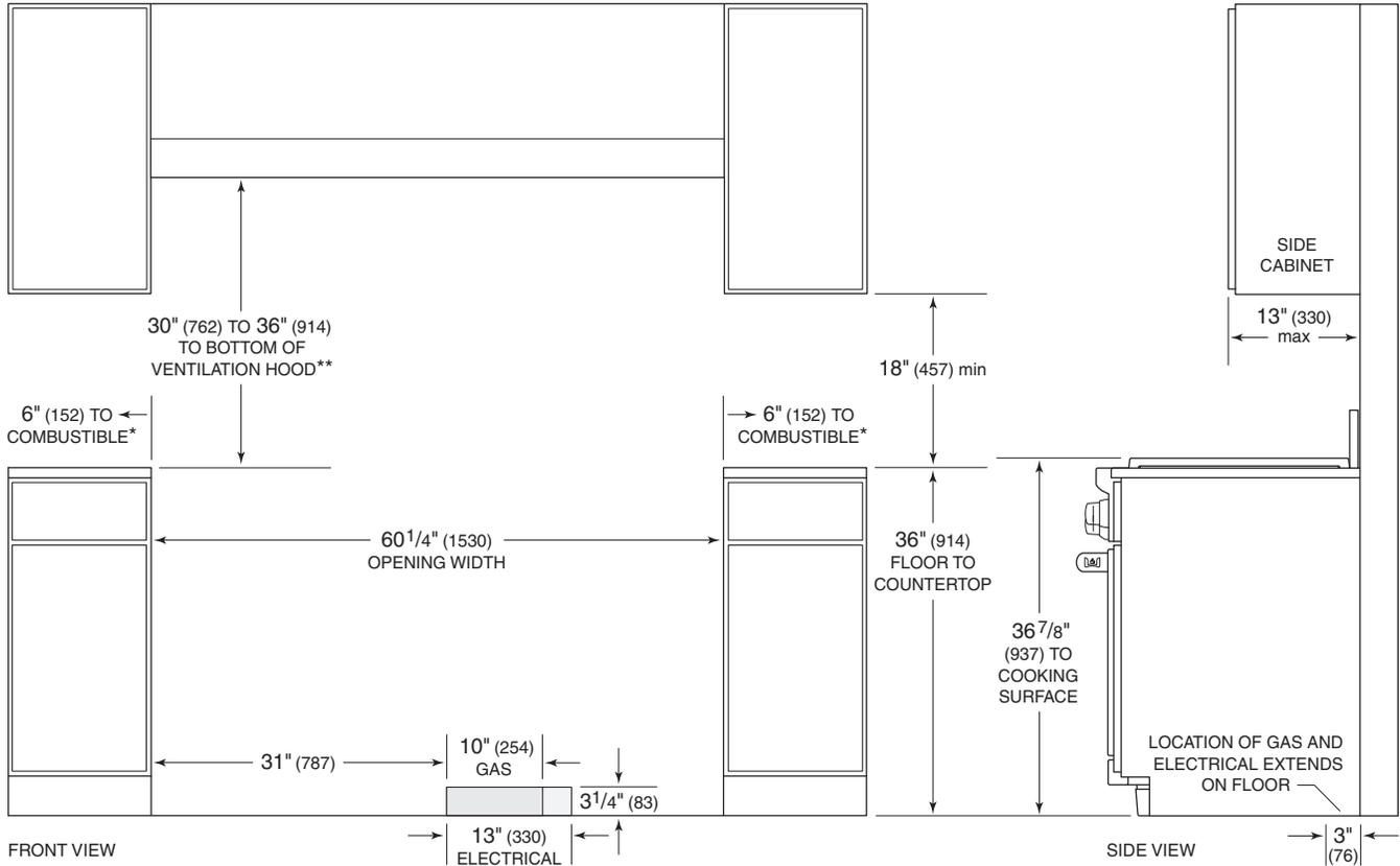
\*Minimum clearance from rough opening to combustibile materials up to 18" (457) above countertop.
