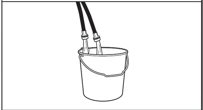
Run water for a few seconds through hoses into a laundry tub, drainpipe, or bucket to avoid clogs. Water should run until clear.
