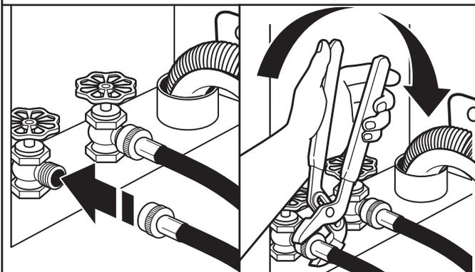
Attach hose to hot water faucet. Screw on coupling by hand until it is seated on washer. Use pliers to tighten couplings an additional 2/3 turn. Repeat this step with second hose for cold water faucet.
