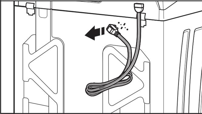
Firmly grasp power cord plug and pull to free from rear panel. Gently place power cord over console to allow free access to back of washer.
