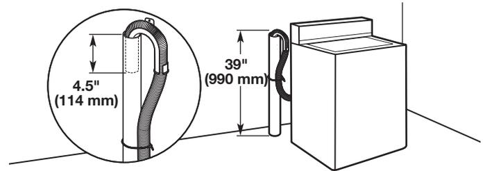
Minimum diameter for a standpipe drain: 2" (51 mm). Minimum carry-away capacity: 17 gal. (64 L) per minute. Top of standpipe must be at least 39" (990 mm) high; install no higher than 96" (2.44 m) from bottom of washer. If you must install higher than 96" (2.44 m), you will need a sump pump system.
