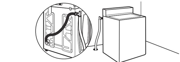
Floor drain system requires a Siphon Break Kit (Part Number 285834), two Connector Kits (Part Number 285835), and an Extension Drain Hose (Part Number 285863) that may be purchased separately. To order, please see toll-free phone numbers in your Use and Care Guide. Minimum siphon break: 28" (710 mm) from bottom of washer. (Additional hoses may be needed.)
