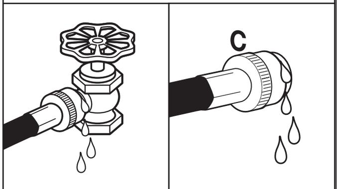
Turn on water faucets to check for leaks. A small amount of water may enter washer. It will drain later.
