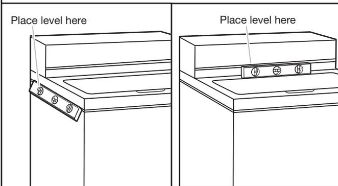
Move the washer to its final location. Place a level on top edges of washer. Use side seam as a guide to check levelness of sides. Check levelness of front using lid, as shown. Rock washer back and forth to make sure all four feet make solid contact with floor. If washer is level, skip to step 3.
