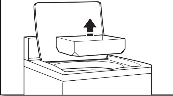
Remove tape from washer lid, open lid, and remove cardboard packing tray from tub. Be sure to remove all parts from tray.
