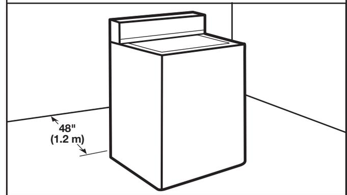
Move washer to within 4 ft (1.2 m) of its final location; it must be in a fully upright position.
