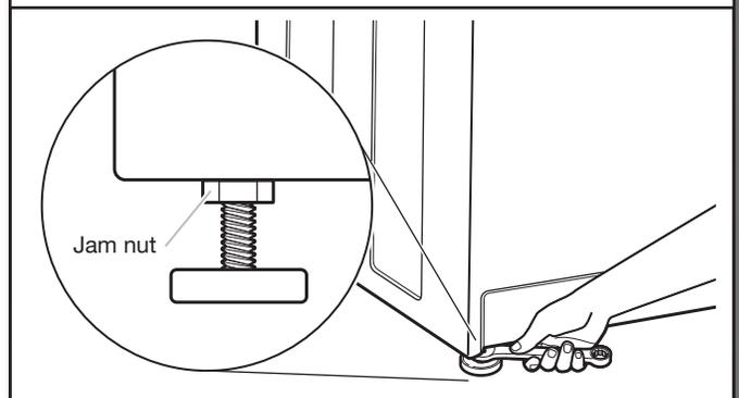
When washer is level, use a 9/16" or 14 mm open-end or adjustable wrench to turn jam nuts counterclockwise on leveling feet tightly against washer cabinet.
