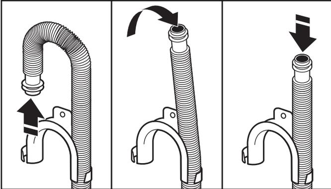
For floor drain installations, you will need to remove the drain hose form from the end of the drain hose. You may need additional parts with separate directions. See “Tools and Parts.”
