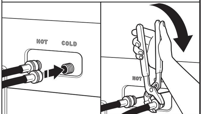
Attach hot water hose to hot water inlet valve marked with a red ring. Screw coupling by hand until it is snug. Use pliers to tighten couplings an additional 2/3 turn. Repeat with cold water inlet valve.
