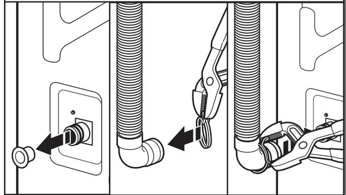
Remove the red plastic plug from the black drain port on the back of the washer.
