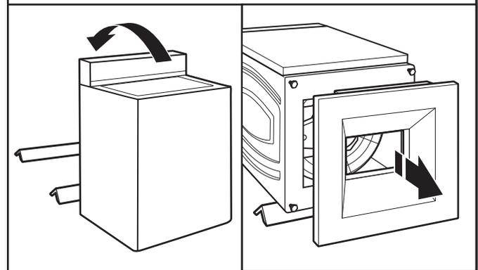
To avoid damaging floor, place cardboard supports from shipping carton on floor behind washer. Tip washer back and place on cardboard supports. Remove shipping base. Set washer upright.
