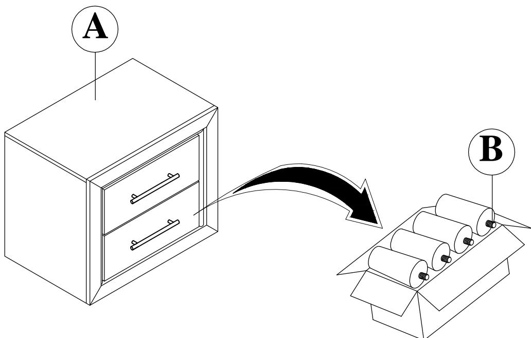
**STEP 2 :** Place the Nightstand (A) upside down on a clean and flat surface. Assemble the Leg (B) with Nightstand (A) by twisting each leg into the corresponding hole until securely tightened.
