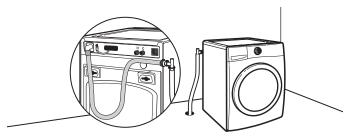
Floor drain system requires a Siphon Break Kit (Part Number 285834), 2 Connector Kits (Part Number 285835), and an Extension Drain Hose (Part Number 285863) that may be purchased separately. See "Alternate Parts". Minimum siphon break height: 28" (710 mm) from bottom of washer. Additional hoses may be needed.
