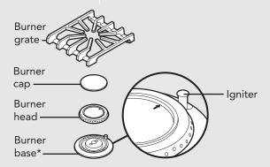
\*Note: When replacing burner head, arrow must be pointing towards back of rangetop.
