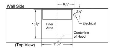
A minimum of 25 sq. in. of exhaust opening space per blower/filter assembly, located above the filter assembly outlet (top), is required for proper air recirculation.
