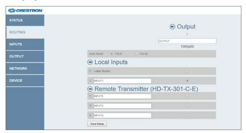
As shown above, the Routing page of the HD-MD switchers contain an **Output** section in the upper-right corner of the page, an option to enable or disable automatic routing (Auto Route), a Local Inputs section, and a Remote Transmitter (HD-TX-201-C-2G-E or HD-TX-301-C-E) section.
