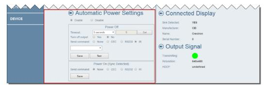
By default, automatic power-off and power-on settings are disabled (the **Disable** radio button is selected). To enable automatic power settings, click the **Enable** radio button. For configuration information, refer to "Configuring Power-Off Settings" and "Configuring Power-On Settings" that follow.
