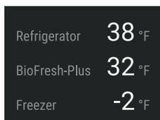
The temperature display blinks if the actual interior temperature is different to the target temperature. It stops blinking when the target temperature is reached.
