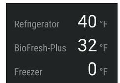
The refrigerator temperature display flashes if the actual refrigerator temperature is different to the target temperature. It stops flashing when the target temperature is reached.
