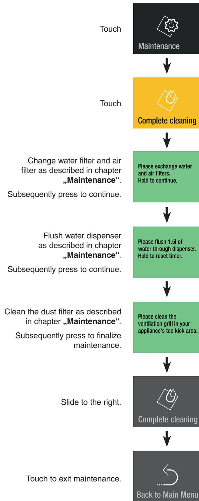
Obtain water filter and air filter from your dealer and complete the maintenance procedure.
