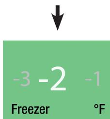
The number flashing at the bottom right shows the actual interior temperature. It disappears when the target temperature is reached.
