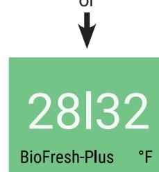
An additional drawer divider must be inserted to select 28°F / 32°F.
