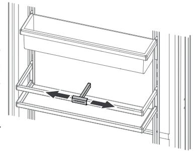
Move the bottle holder to the desired position. Always hold at the front when moving.
