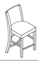
Do not fully tighten any bolts until last step
