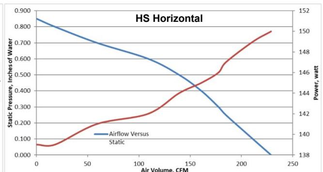
\*When configured for outside ventilation. Independently tested through the AHAM Verified program.
