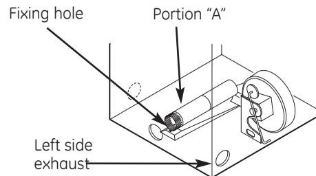
Reconnect the cut portion (A) of the duct to the blower housing. Make sure that the shortened duct is aligned with the tab in the base. Use the screw saved previously to secure the duct in place through the tab on the appliance base.
