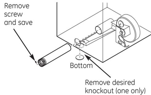
Remove the screw inside the dryer exhaust duct and save. Pull the duct out of the dryer. Detach and remove the bottom knockout.
