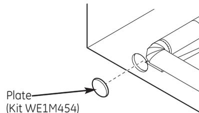
Connect standard metal elbows and ducts to complete the exhaust system. Cover back opening with a plate (Kit WE1M454) available from your local service provider. Place dryer in final location.
