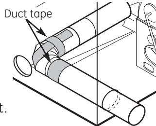
**⚠ CAUTION:** Internal duct joints must be secured with tape; otherwise, they may separate and cause a safety hazard.
