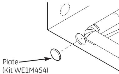
Connect standard metal elbows and ducts to complete the exhaust system. Cover back opening with a plate (Kit WE1M454) available from your local service provider. Place dryer in final location.
