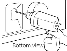
**NOTE:** Make sure the hole is drilled all the way through the elbow and pipe.
