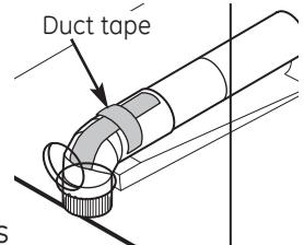
**NOTE:** Make sure the tape covers the screw hole in portion A where it connects to the elbow.
