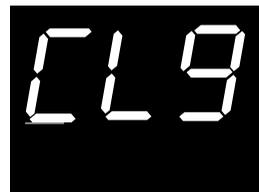
If you observe "CLg" in the display window you must clean your exhaust ducting before you complete installation. Check exhaust ducting for obstructions or blockages, especially around turns. Contact a qualified service provider if necessary.
