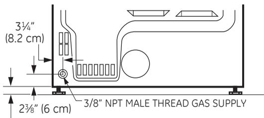
**NOTE:** Add to vertical dimension the distance between cabinet bottom to floor.
