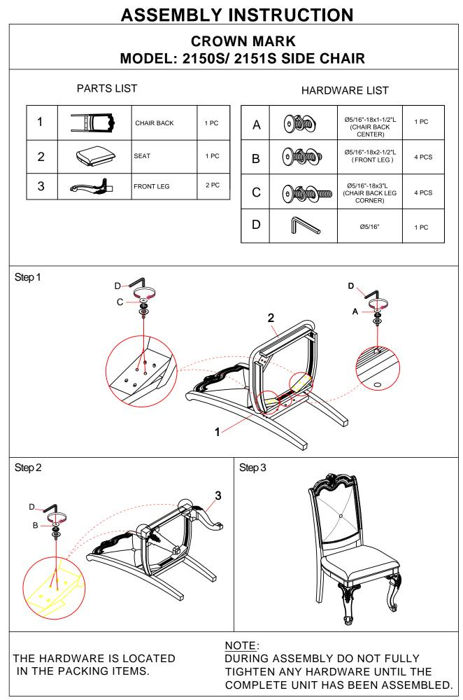
NOTE: MUST TIGHTEN SCREWS PERIODICALLY WITH USE SCREWS WILL BECOME LOOSE. CHECK TIGHTNESS OF ALL SCREWS EVERY 6-8 WEEKS.
