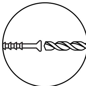
3. Only drill horizontally. Do not force the drill or enlarge the hole for the wall anchor.
