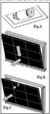
The carbon filters can only retain odours for a limited period of time. They cannot be washed, therefore, it is recommended they are replaced at least once every six months or more frequently in the case of a heavy use of the appliance.
