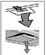
Special attention should be reserved to the metal grease filters. An excess of grease in the filter, as well as affecting the performance of the hood, can also be a fire risk. To avert fires, the filters must be cleaned regularly at least once a month or more frequently, in the case of a heavy use of the appliance.
