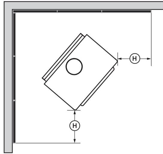
Figure 14: Heat shield clearances
