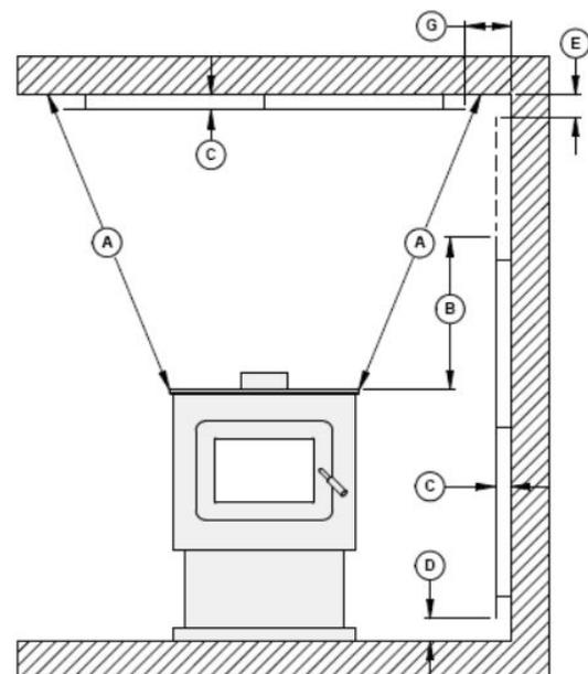
Figure 12: Heat shield clearances
